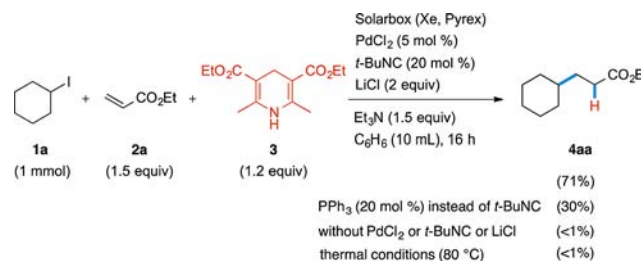
Scheme 2. Photoinduced Reductive Radical Addition of Iodocyclohexane 1a to Ethyl Acrylate 2a
